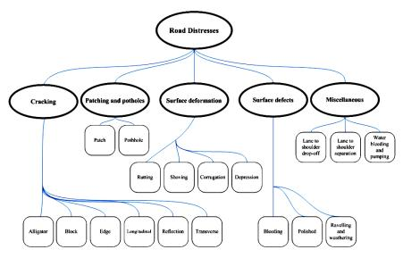
Figure 1 S.H.R.P Asphalt concrete surfaced pavement distress types
