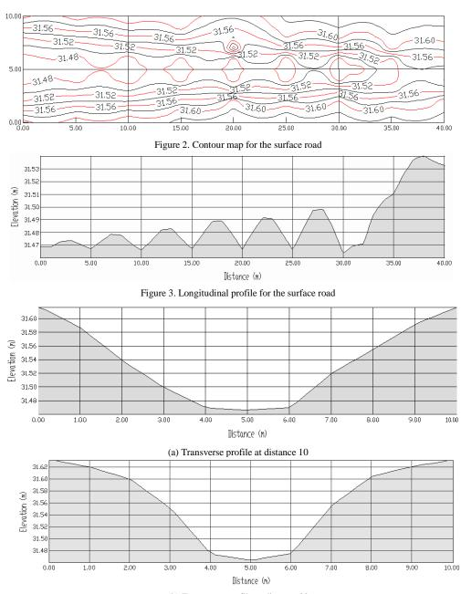
(b) Transverse profile at distance 30 Figure 4. Transverse profiles for the surface road
